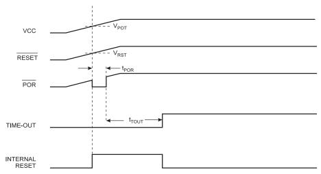
If the build-in start-up delay is sufficient,  $\overline{\text{RESET}}$  can be connected to  $V_{CC}$  directly or via an external pull-up resistor. By holding the  $\overline{\text{RESET}}$  pin low for a period after  $V_{CC}$  has
