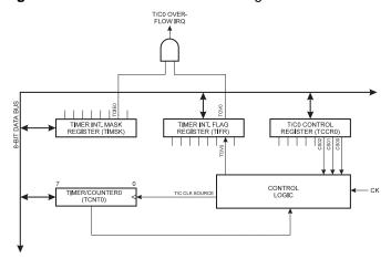
The 8-bit Timer/Counter0 can select clock source from CK, prescaled CK, or an external pin. In addition it can be stopped as described in the specification for the Timer/Counter0 Control Register - TCCR0. The overflow status flag is found in the Timer/Counter Interrupt Flag Register - TIFR. Control signals are found in the Timer/Counter0 Control Register - TCCR0. The interrupt enable/disable settings for Timer/Counter0 are found in the Timer/Counter Interrupt Mask Register - TIMSK.
