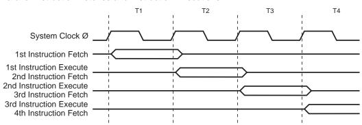
Figure 12 shows the internal timing concept for the register file. In a single clock cycle an ALU operation using two reg-
