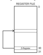
The register accessed is the one pointed to by the Z-register (R30).
