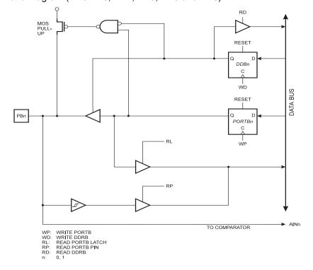
Figure 29. Port D Schematic Diagram (Pin PD2)
