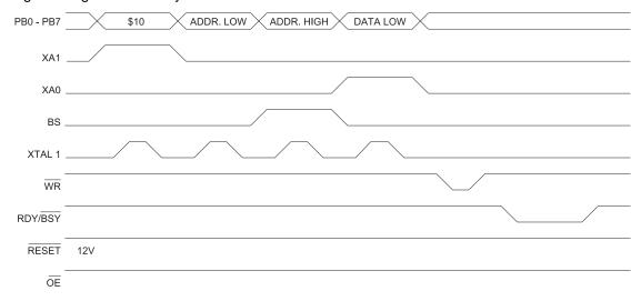
Figure 33. Programming Flash High Byte
