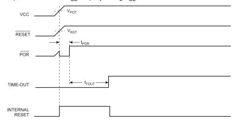
Figure 15. MCU Start-Up, RESET Tied to V<sub>CC</sub>. Slowly Rising V<sub>CC</sub>
