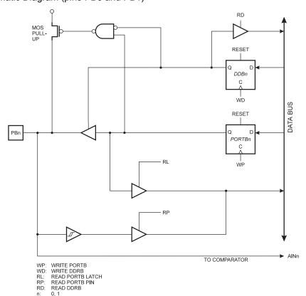
Figure 24. Port B Schematic Diagram (Pins PB2, PB3 and PB4)
