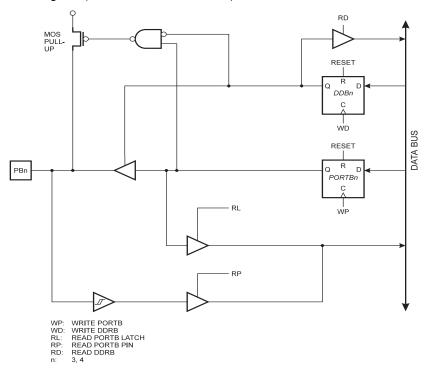
Figure 25. Port B Schematic Diagram, Pin PB5
