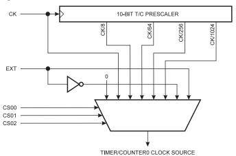
The four different prescaled selections are: CK/8, CK/64, CK/256 and CK/1024 where CK is the oscillator clock. For the Timer/Counter, added selections as CK, external source and stop, can be selected as clock sources.
