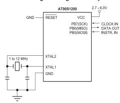
When writing serial data to the AT90S1200, data is clocked on the rising edge of CLK.
