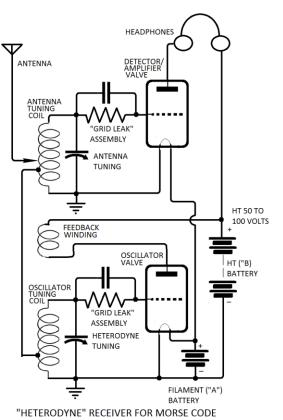
became available, it was more practical a single to use carrier frequency, and have a valve-"local" based oscillator to provide the heterodyne signal at the receiver. This also allowed operators to adjust the pitch to their suit own preferences. (Nowadays this is referred to as a "Beat Frequency Oscillator or "BFO"). had Operators noticed that if the
