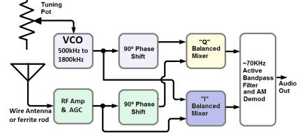
With a dual quadrature mixer, it can be configured so that the only output signal frequency is the incoming signal frequency subtracted from the oscillator frequency. So 1.07MHz - 1.0MHz = 0.07Mhz (70 kHz), which is what we want, but as for the image frequency, we get 1.07MHz - 1.14MHz, which comes out as *minus* 70kHz!
