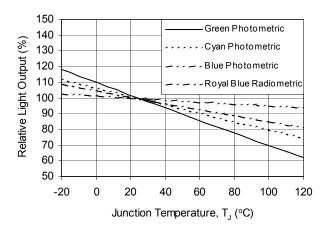
Figure 2. Relative Light Output vs. Junction Temperature.
