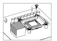
3. Insert the four plastic push pins into the hole of the plastic insert.
