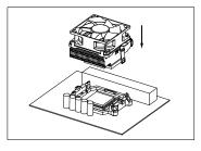
C) Install the cooler by pressing the mounting clip until it's hooked in.
