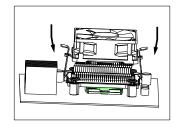
5. Install the cooler by pressing the mounting clip until it's hooked in.
