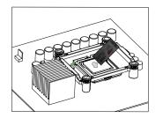
4. Apply the thermal compound on the surface of CPU metal plate.
