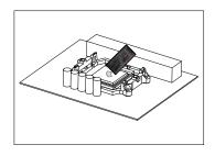
B) Place the cooler on top of the CPU.
