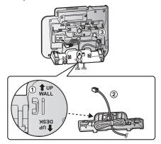
3 Insert the lower tabs of the adaptor into the unit's bottom slots (1), then insert by pushing
