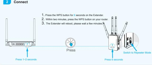
Tips:The corresponding WLAN LEDs should turn on and stay solid, indicating successful connections.
