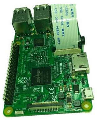
Gently press the grey tabs back down (both at the same time) to lock the ribbon cable in place.
