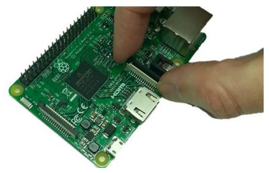
Open the 5MP Camera, and insert the end of the ribbon cable into the camera socket, with the metal contacts facing towards the HDMI socket.
