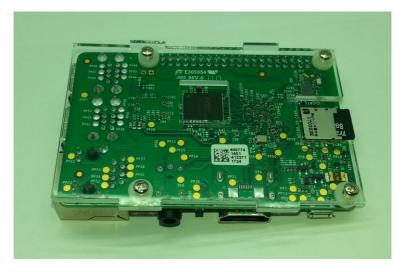
Attach the bottom plate to the Raspberry Pi, noting the slots for the main processor IC and MicroSD card slot. The insulating washers sit between the plate and the board.
