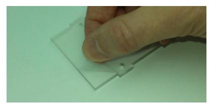
Start by carefully removing the protective film from all the acrylic pieces. You might find that gently scratching the corner with a fingernail will help to start the process.
