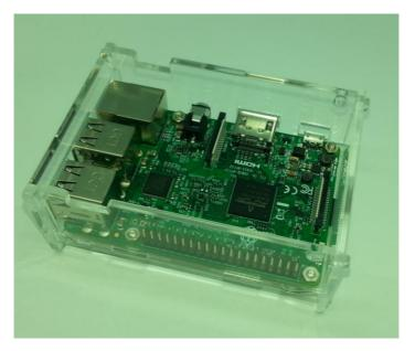
Attach the fourth side (with slot for MicroSD card) by clipping it into the other three sides, again gently squeezing the lower tabs if necessary.
