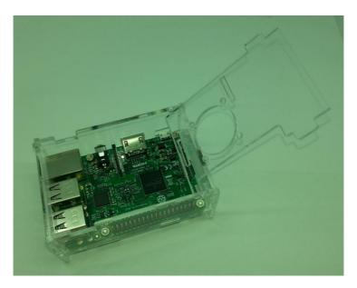
Assembly of the case takes a bit of care to ensure all the parts are oriented correctly, but is otherwise fairly straightforward. We would recommend having a small Philips screwdriver and pliers to fasten the nuts and bolts.
