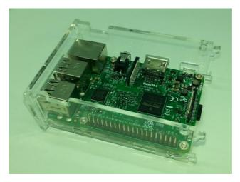
Place the above assembly around the Raspberry Pi and line up the slots.
