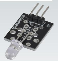
Infrared Transmitter Module
