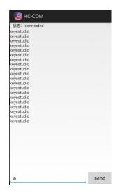
Open APP HC-COM, click search device, select the device, device is connected; the LED on the Bluetooth module is on. Enter "a" in HC-COM, click send, Bluetooth APP will display keyestudio. Every time HC-COM sends an "a", the Pin13 LED on the main board blinks once.
