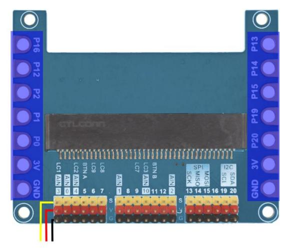
To use the sensor shield adapter, you can either directly plug onto the connections on the board using jumper wires, or via alligator clips on the side of the board.
