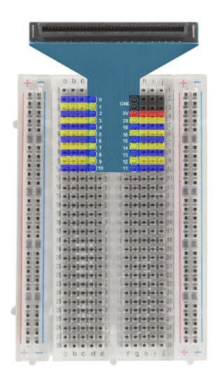
To use the T-type adapter, you can either directly plug onto the connections on the board using jumper wires, or as shown in this example we have mounted the XC4334 onto a breadboard from our range (PB8820).
