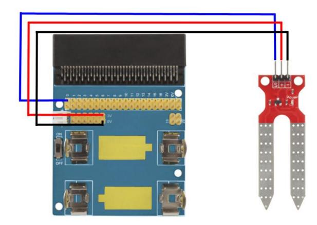
The XC4330 module is perfect for creating portable projects. This example uses our soil moisture module to create a handy pocket soil moisture meter for checking plants in the garden.
