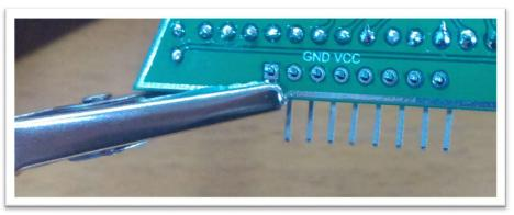
Here, we'll hold it from the left, and solder the right most connection, just to hold it in place. Make sure that the alligator clip is not bending the component or putting it in an awkward position; this too can take a bit of practise.
