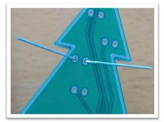
Once that is done, you will want to snip the legs of the LED much shorter. We do this so that the heat from the soldering iron is not wasted heating up the whole leg, only the small section close to where we want to solder
