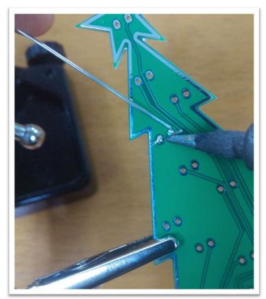
Here, you can see we have the PCB mounted in our "Third Hand" holder, TH1982. We apply the soldering iron to one side of the LED leg, touching both the leg and the pad underneath.
