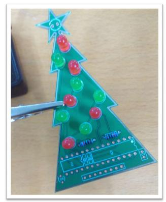
Similar to the LEDs: bend the legs so that they don't move, then snip them down to size. Heat from one side and apply solder from the other side, for each joint on the underside of the PCB.
