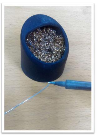
When preparing the iron, and it is sufficiently hot enough to melt solder, you want to touch the solder onto the iron itself, so that the solder and flux (a component of the solder responsible for keeping the joint clean and flowy) cleans any rust or dirt off the tip of the iron.
