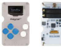
**Please Note:** The holes of acrylic bottom board should be aligned with the potentiometer on the console when installing it.
