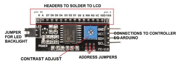
*Please note, the white mark separating the first/last pin can appear on either side but is unimportant to the layout.*
