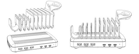
The tabs on the plastic divider are inserted into the upper groove of the charging module. The width can be freely adjusted from left to right according to the size of the device.
