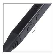
**2.** Click the filament loading button once to start heating. When the actual temperature reaches the preset temperature, the pen is ready to work.
