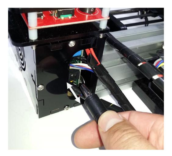
Power up unit via wall socket adaptor.
