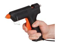
2. Press the trigger gently until resistance is felt to ensure the glue stick is installed correctly
