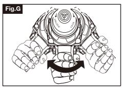
⚠ WARNING: Never change the direction of rotation when the chuck is rotating, wait until it has stopped!
