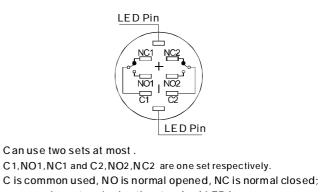
+  $\ensuremath{{\scriptstyle -}}$  are lamp terminals, the standard LED have no difference of anode and cathode;
