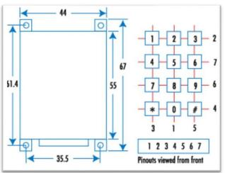
This style of setup is most often called a "matrix keypad" and each of the keys forms a bridge or short across two of the corresponding pins. For example, if you were to press the number "5" on the keypad, there would be a connection between pins 1 and 7 on the row.
