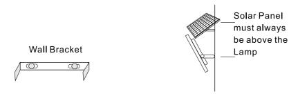
Please make sure the Solar panels are installed at the correct Angle for your Country and in the correct direction for your Hemisphere. Also ensure that the sunlight to them is not blocked by obstacles such as trees, shadows, buildings etc. The panel needs unobstructed sunlight to charge correctly.
