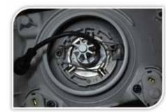
Align the snap ring to install the LED light and place the wire inside
