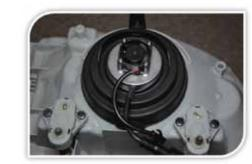
Rotate the LED light gently inside when installing the fan
