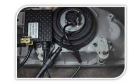
Connect the LED light, fan and the ballast wires together. Place the ballast near the LED light. Note: position may differ depending on the model of the car
