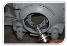
Take out the existing halogen lamp after unlocking it
