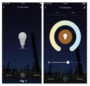
Open the control panel for devices. For example, Fig. 1 shows the light is off, and only the timer can be accessed in the off mode. Fig. 2 shows the light is on, and scene, color, brightness, and schedule can be configured in the on mode. Click".." at the top right corner of the control panel to manage individual devices.
