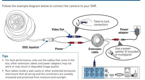
Avoid bending the cable at sharp angles. Too many bends (or Images contained in this diagram are even just one really sharp one) can disrupt the signal to the for illustrative purposes only point of failure.
