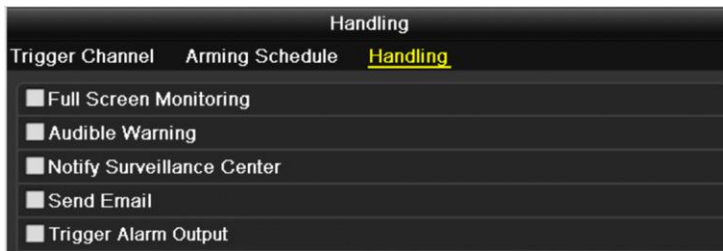
Figure 8.5 Set Alarm Response Actions of Motion Detection
