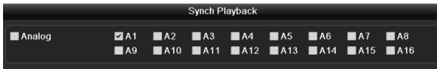
Figure 6.12 Select Channels for Synchronous Playback
