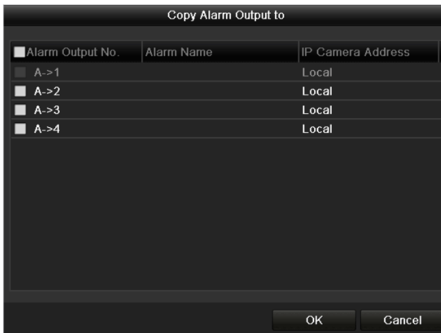
Figure 8.19 Copy Settings of Alarm Output
