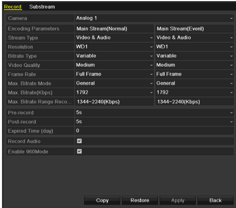
Figure 5.3 Encoding Parameters-Main Stream
