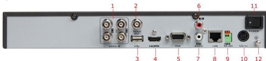
Figure 1.5 Rear Panel of 4CH DVR
