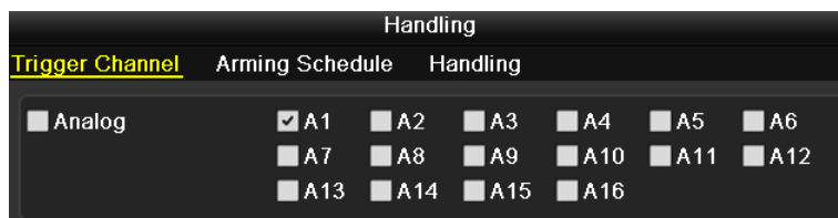
Figure 8.3 Set Trigger Camera of Motion Detection
