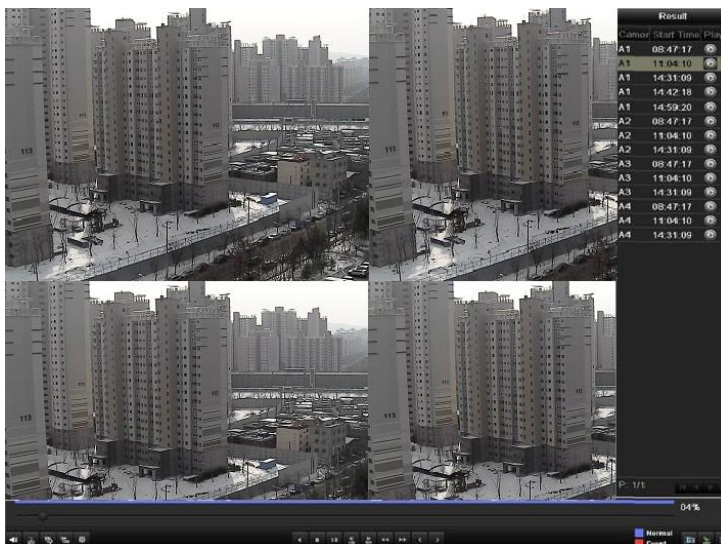
Figure 6. 14 4-ch Synchronous Playback Interface with Video List
