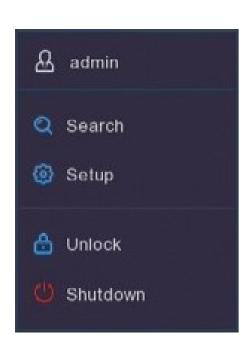
In this menu you can switch users, search videos, set up your DVR/NVR, manually lock the screen and shutdown, reboot or logout of the system.
