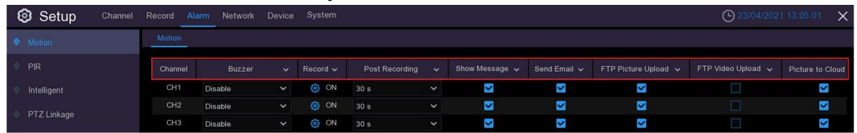
Channel: Channel number being setup.
