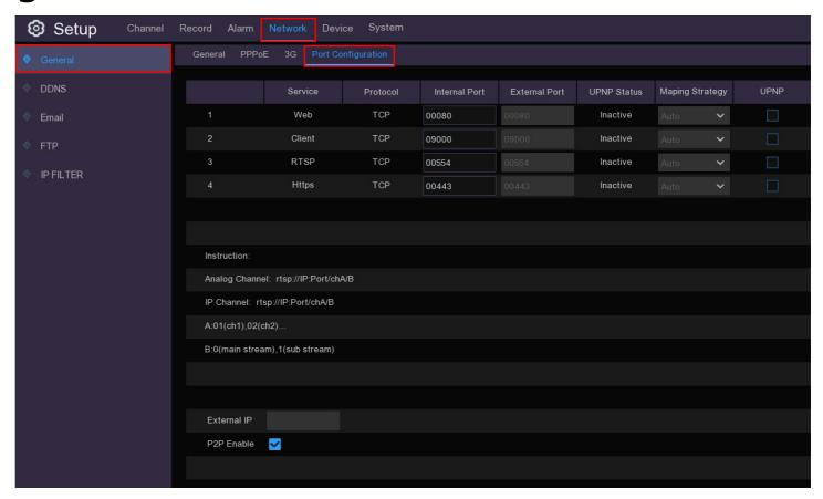
**UPNP:** If you want to log in remotely to the DVR using the Web Client, you need to complete the port forwarding. Enable this option if your router supports the UPnP. You need to enable UPnP both, on DVR and router, this will need to be done manually. If your router does not support UPnP, make sure the port forwarding is completed manually.
