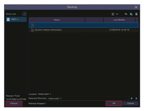
**8**. If you are unsure whether your USB storage is correctly formatted click the Format button. Check the directory to make sure the video is being saved to the correct location and click OK. The system will automatically assign file names to your video clips.
