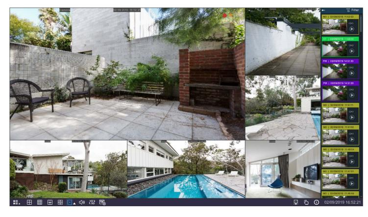
The Live View screen is the default display you will see when the DVR is on. You will be able to see each of the connected cameras and you can select the format in which they are displayed with either single images, scrolling single images or multiple images on the one screen.
