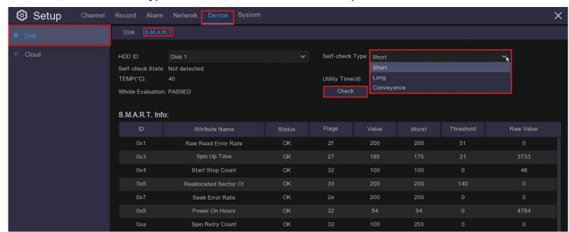
**Conveyance**: This is a very quick test that verifies the mechanical parts of the hard drive are working.
