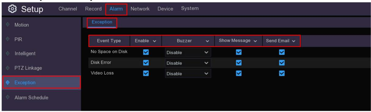
**Event Type**: Your DVR can be set to alert you if it runs out of HDD space (No Space on Disk), there is an error on the HDD (Disk Error) or if one or more cameras have stopped sending a signal to the DVR (Video Loss).
