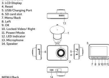
Press MENU/2 button to enter Menu selection during standby mode, to press the back button to back to the video standby mode.
