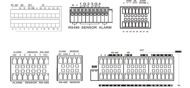
**Alarm input:** Check your purchased alarm device and connect a G (GND) foot to the port marked with "-" and connect the alarm channel to the port marked with "+".
