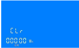
Figure 9 clear the energy interface
