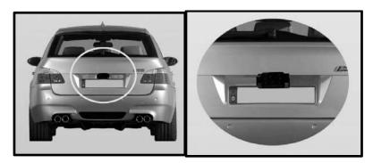
1. Remove the rear license plate, and then loosen the bolts/screws of the license plate.
