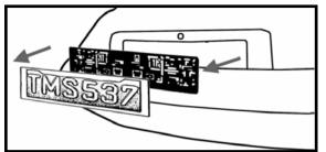
2. Position the mounting plate of the camera behind the license plate bracket. Secure both license plate bracket and mounting plate with the license plate bracket bolts/screws.
