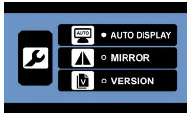
Auto Display; this setting allows you to set your main view. The selected camera (CAM1 or CAM2) will be displayed automatically when backing up. In order to show the picture of both cameras at the same time, please SPLIT in the menu (only if both signals can be received – otherwise the monitor will show the available picture in full screen).
