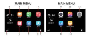
Touch the icon on the desired mode on screen and the unit will then enter into the mode that selected for operation. Hold & slide on screen to shift to other **MAIN MENU** that shows the hidden input or operation icons.
