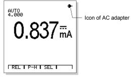
Turning off the meter, when using AC adapter to supply power, the meter will return to charge function until the AC adapter is unconnected. So, to make the meter turned off completely, the AC adapter would be cut off.
