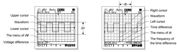
The cursor readout function is effective only when the waveform is frozen (by HOLD or single trigger). After the waveform frozen, press F4 to enter the Cursor Readout sub-menu:
