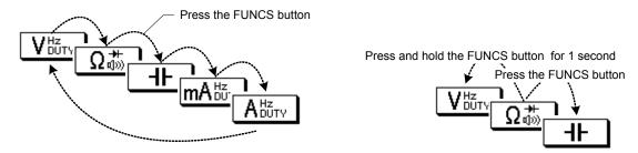
Each time the button FUNCS pressed, the next function will be selected in that order. To select the function inverse the order, press and hold the button for 1 second.
