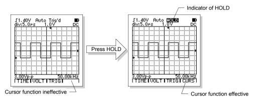
The key of **HOLD/MEM** can start and stop waveform acquisition. When the instrument has stopped acquiring waveform data, the display is frozen.
