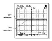
Zero-volt waveform is 6 points below the vertical zero reference.
