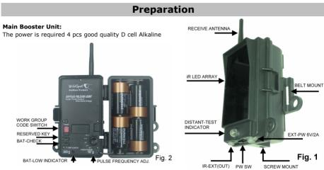
batteries for the best result in operation. Do not try to mix old and new batteries together. After installing batteries according to the polarity mold on the cabinet into the compartment, push the **BAT-Check** button once and see if the Bat-Test LED does work in order to verify the battery polarity to be correctly. (**Fig. 2**)
