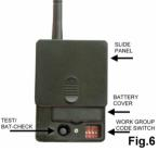
After finish self-test, remember to slide the PW switch to OFF (At Center)
