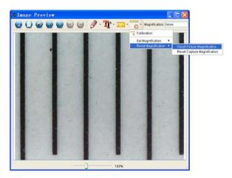
2. Change the magnification rate and capture several pictures, click on the picture to enter into measurement
