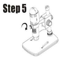
Rotate Wheel 11 clockwise to fix the microscope on the ring.
