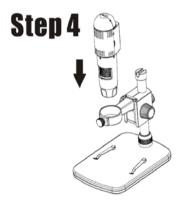
Put the microscope into the ring of the stand!
