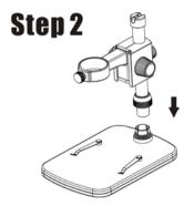
Put the metal pole into the female part of the stage!
