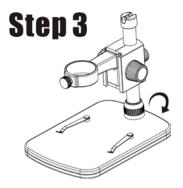
Rotate Wheel 10 to fix the pole on the stage!
