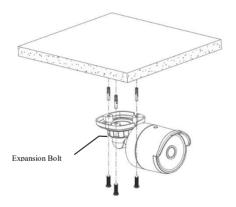
Insert three expansion bolts in place into the ceiling and fix the equipment with three locking screws.
