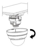
After angle adjustment, mount the shield back by rotating the collar up.
