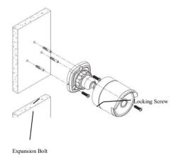
Insert three expansion bolts in place into the wall and fix the equipment with three locking screws.
