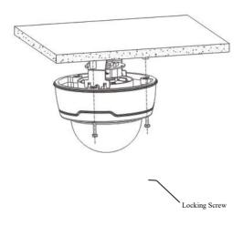
Fix the front component on the pedestal by tightening the three locking screws.
