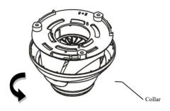
Remove the collar off the camera by rotating it down
