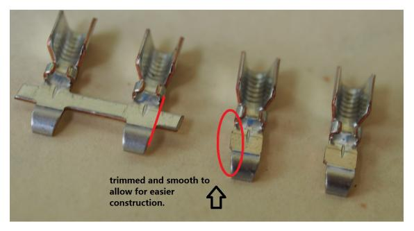
The metal connectors can then have the lead connected and be pushed through the plastic housing, in which they should "click" into place, with the metal lip facing downwards to latch over the thin metal in the housing.
