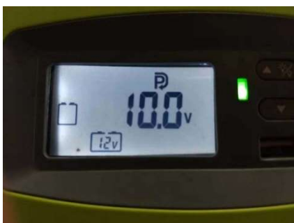
Battery low voltage protection setting
