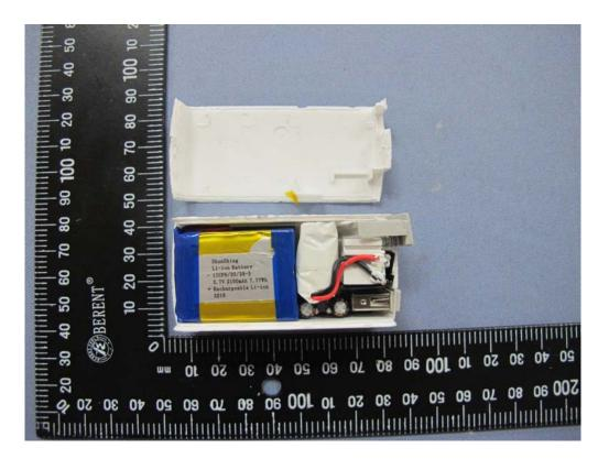
Figure 3 Internal view of power bank
