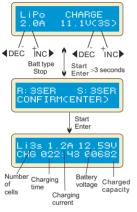
The left side of the first line shows the type of battery you choose. The value on the left of the second line of the charger is current user set. After setting the current and voltage, press START/ENTER key for more than 3 seconds to start the process.(charge current: 0.1-5.0A, voltage: 3.7-22.2V).
