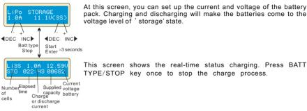
At this screen, you can set up the current and voltage of the battery pack. Charging and discharging will make the batteries come to the voltage level of 'storage' state.
