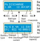
Set up the charge current on the left and nominal voltage on the right. Range of discharge current is 0.1-1.0A, the voltage should match the battery being charged. Press START/ENTER key for more than 3 seconds to start charging.
