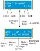
Set charge current on the left and the final voltage on the right. Range of the charge current is 0.1-1.0A; range of final voltage is 0.1-25.0V. Press START/ENTER key for more than 3 seconds to start the program.
