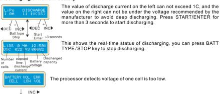
The 4th cell was damaged. The value of voltage may be zero if disconnection occurs.
