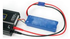
The main battery leads must be connected along with the balance lead connector as shown before charging your battery ..
