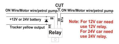
**Attention:** Turning off engine is very dangerous when car is driving, this will make the car difficult to control and maybe cause a accident, so we recommend connect the relay to cut the start motor wire, this will make driver can not remote turn off car engine, but can not start car engine.
