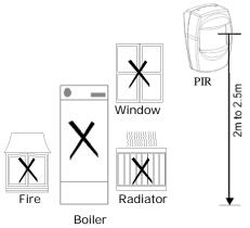
detected. To overcome this it is recommended that the pets are kept in one specific room out of sight of a PIR when the system is armed. If required, additional MC (available as accessories) can then be used to protect the doors and windows of the room
