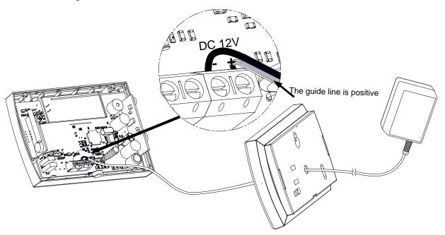
**CAUTION**: To avoid the risk of electrical shock you must always totally isolate the mains supply before opening the control panel cover(s).
