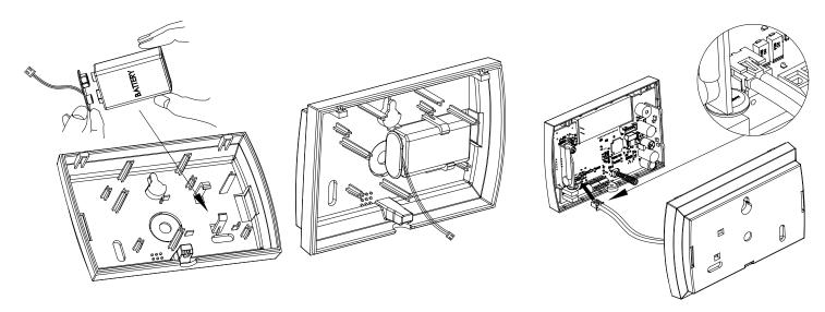
b. Fit the cover to hold down the tamper spring at the bottom right-hand of the board.
