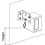
Step 4: set Infrared Beam and reflector in the same level
