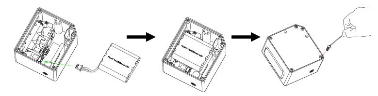
**Step 3:** fix Infrared Beam , use fixing panel ;then set fixing panel fix to the wall; fixing height by yourself demand (height from 30 to 120cm )
