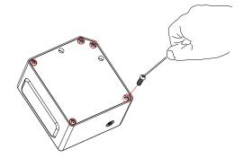
**Step 2:** Place  $4 \times 1.2V$  batteries pack inside the battery compartment with the correct polarity and then close the base cover and screw it up.
