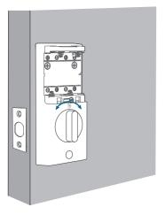
Make sure the deadbolt is retracted and the thumb turn knob is on the 'unlock' position, check if the deadbolt moves properly by turning the thumbturn.
