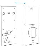
2. Run the wires through the back cover.
