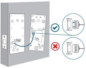
5. Mount the interior assembly. Make sure both wires are tucked into the cabin on the back of the interior assembly.
