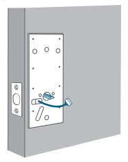
3. Secure the back cover with screws.
