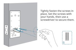
• (Optional) If the back cover is not fastened tightly to the door, use the additional screw provided.
