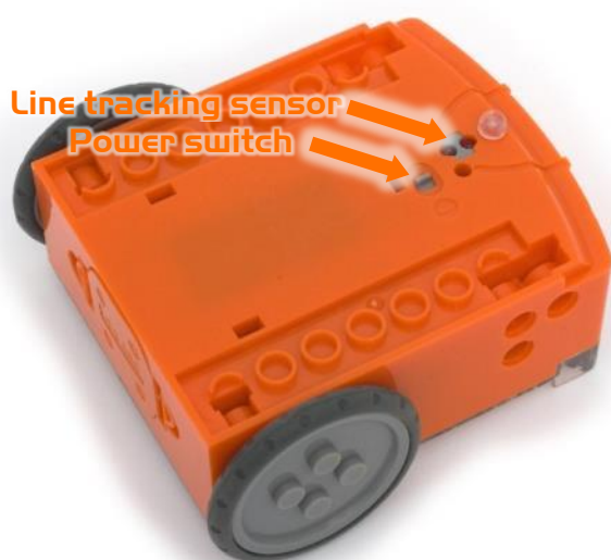
Edison's power switch and line tracking sensor
