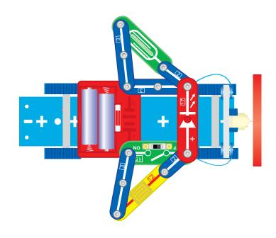
(In 29-34, turn the motor round, you can change the running direction of the vehicle and boat. Also replace the slide switch 15 with the dry reed switch 13 and they will change into a magnet-controlled electric vehicle and boat.)
