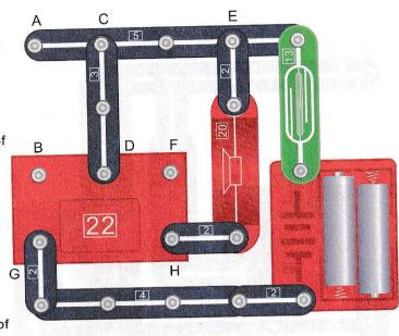
**52.Magnet-controlled sound of vibration**Connect terminal AB and FH,put a magnet near to dry reed switch (3), the speaker (20) will give out sound of vibration.
