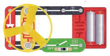
18. An LED and an electric fan connected in parallel. Close the slide switch 15, the red LED 17 will light up and the fan will begin to rotate.
