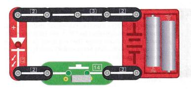
33. Simple and easy signalling practice. Press the press switch 14 rhythmically; the red LED 17 will flash, so it can be used for sending messages in Morse code or make up your own code!
