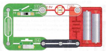
37.Three series connected switches to control a lamp After connecting circuit, you must close the slide switch press the press switch and put a magnet near to dry reed switch press the lamp will light up.
