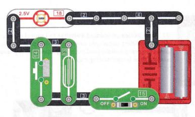
40. This circuit uses two switches in series with one switch in parallel to control a lamp or other device(2). The lamp 18 can be switched on by closing slide switch15, or by closing both switches 13 and 14 at the same time.
