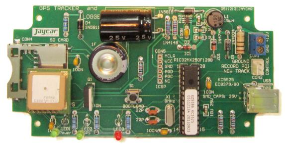
All the parts mount on a single PCB. The GPS module can be seen sitting over the SD card socket on the left, the power supply is on the top right of the board and at the far right are the connectors for power, the optional inputs and the USB socket.
