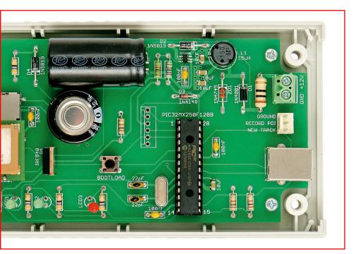
This close-up view shows how the UP501 GPS module and the three LEDs are mounted. The LEDs must be 20mm proud of the PCB so that they protrude through the case lid.
