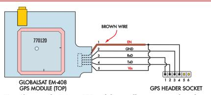
Fig.7: if you use the EM-408 GPS module, cut off one connector from the supplied cable and then solder the cable to a 6-pin header as shown here. This header is then plugged into the GPS header socket on the PCB.
