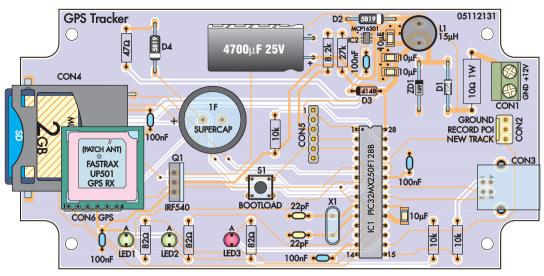
Fig.6: follow this parts layout to build the PCB (note: if you are using the EM-408 GPS module, you can leave out D4, the  $47\Omega$  resistor and the supercap). The completed assembly is mounted in the bottom of the case, with the three LEDs at bottom left protruding through holes drilled in the lid.
