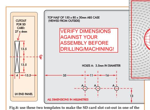
end panels of the case and to drill the holes for the LEDs in the lid.
