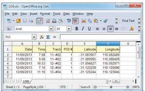
Fig.1: the GPS Tracker can be configured to record POI (point of interest) locations in a spreadsheet called LOG.XLS which makes them easy to reference later on.
