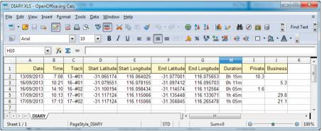
Fig.2: for the tax man, the GPS Tracker can also be configured to record a travel diary in another spreadsheet called DIARY.XLS. In this mode, a trip is deemed to be for business if the POI button is pressed during the journey.
